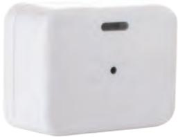
GB-540 is a smart ZigBee wireless two-way acoustic glass-break detector that incorporates advanced algorithms that help reduce a wider range of threats and deliver superior false alarm immunity. Designed to be installed on any interior wall or ceiling to detect the breaking of framed glass, the GB-540 is capable of covering large areas and multiple openings.
